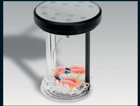
3 The thus prepared denture is fixed with a rubber band at the bracket and then contacted to the plating head.
