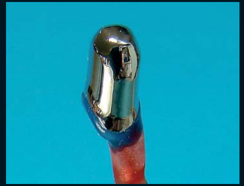
3 The primary part was connected with the magnetic optiCLIC contact stick. Galvanowax was applied up to the preparation margin.
